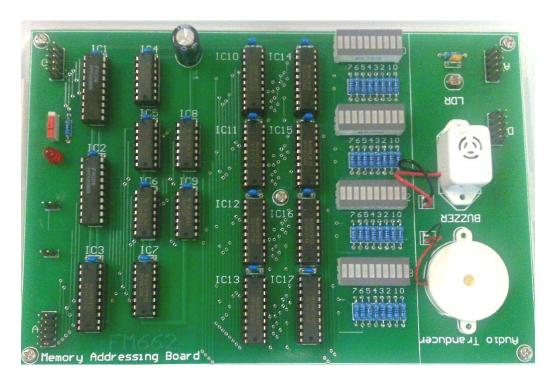
This Peripheral Board is separated into two distinct areas. The larger area on the left (pictured facing the correct way up) is the Memory Addressing Board area. This is used to illustrate how to extend the AVR's limited internal memory by adding external memory. The smaller area on the right (pictured upside-down) is the Sensor/Actuator Board area. This is used to illustrate how to communicate with sensors and actuators using analog and PWM signals.
