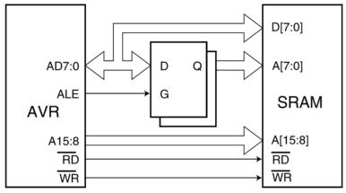
A 16-bit bus is used to communicate the Address & Data busses. These use Ports A & C. In addition, there are three signals, shown on the connector diagram below.
